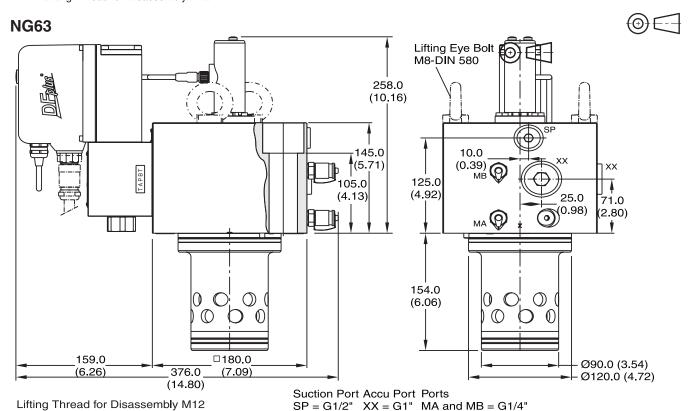
○ Kit Bolt Kit - III F DIN912 12.9 NG Nitrile Fluorocarbon 50 BK513 4 x M20x120 DIN 912 12.8 553 Nm (407.8 lb-ft.) SK-TDP050EN SK-TDP050EV 63 BK420 4 x M30x140 DIN 912 12.9 1910 Nm (1408.6 lb.-ft.) SK-TDP063EN SK-TDP063EV
